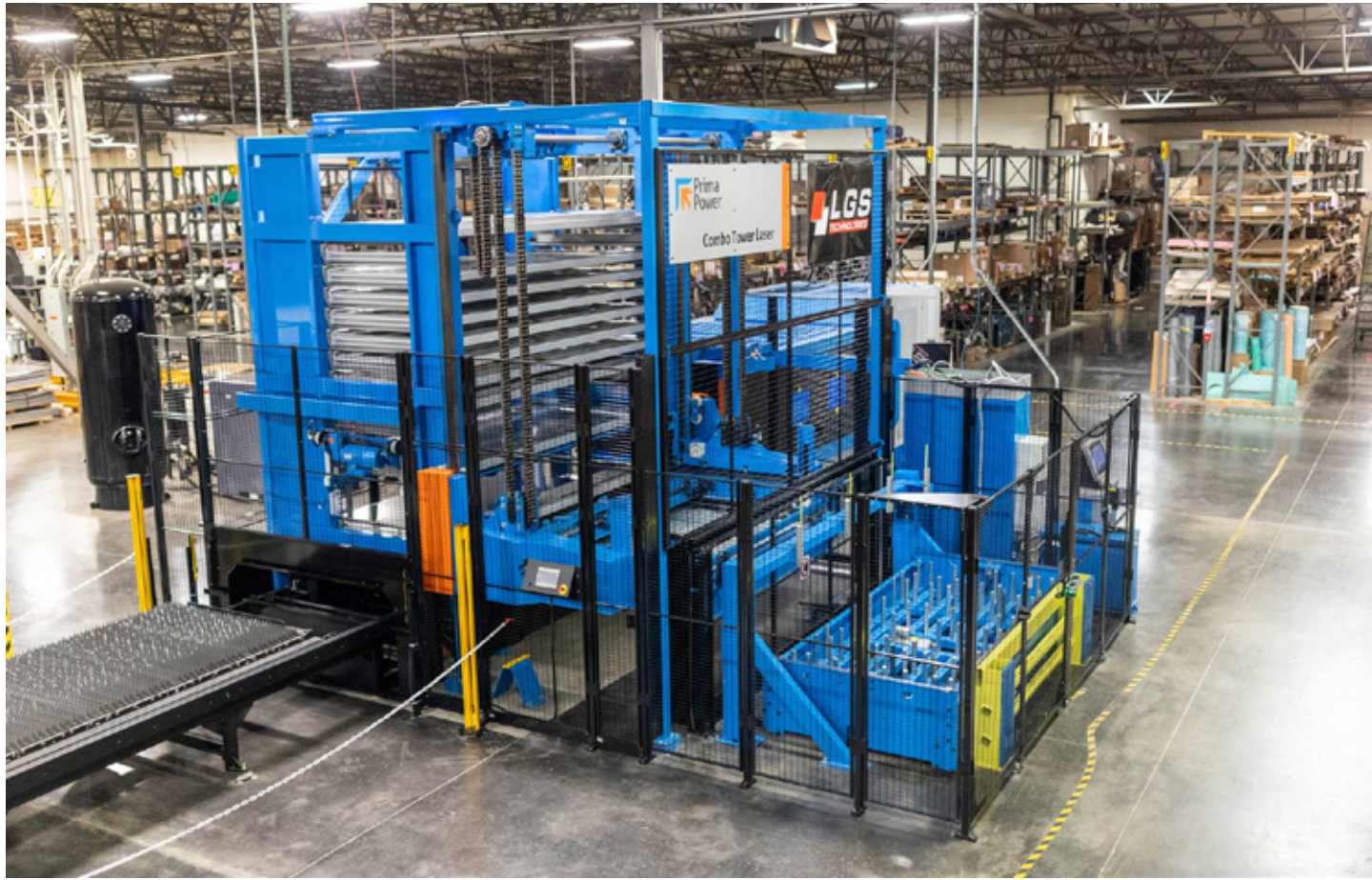
A Prima Power Combi Tower Laser allows LGS Technologies to perform lights-out manufacturing.
