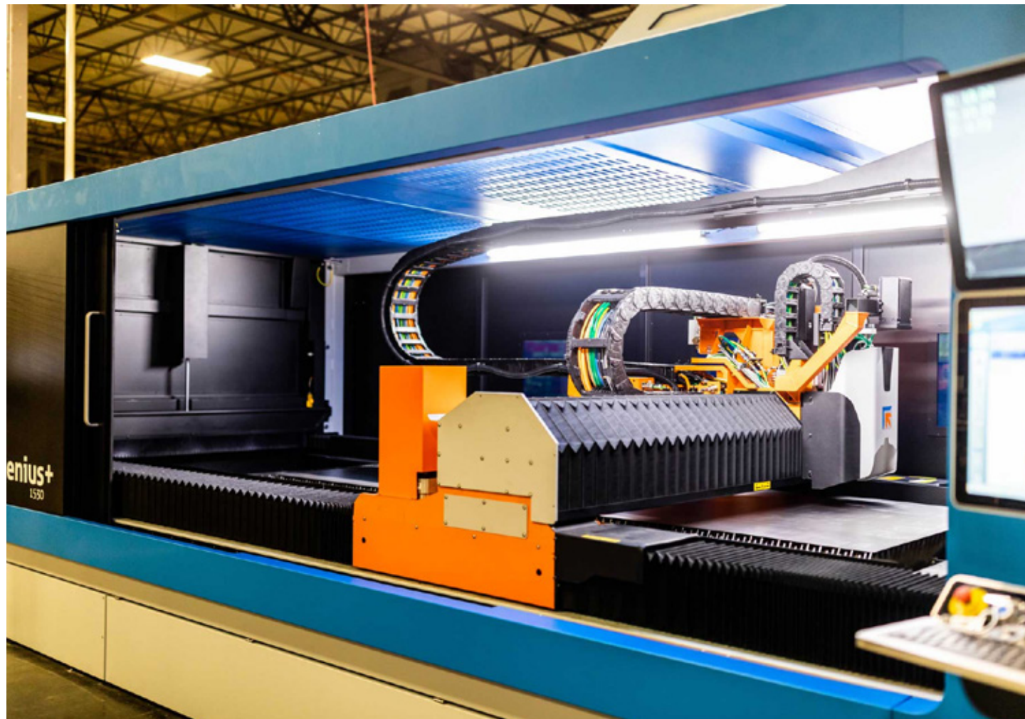
LGS Technologies invested in a Prima Power Laser Genius+ 1530. The 6-kW fiber laser adds versatility and compatibility by processing a range of materials and thicknesses.
